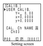
8 Move the cursor using the key and set the value using the numeric pad.
