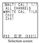
Move the cursor using the key to and select a calibration channel.
